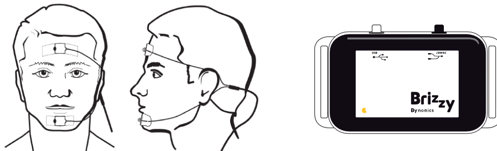
Figure 1: LEFT - Sensor placement for measurement of mandibular movements. RIGHT - Brizzy device for recording of mandible movements during sleep.
